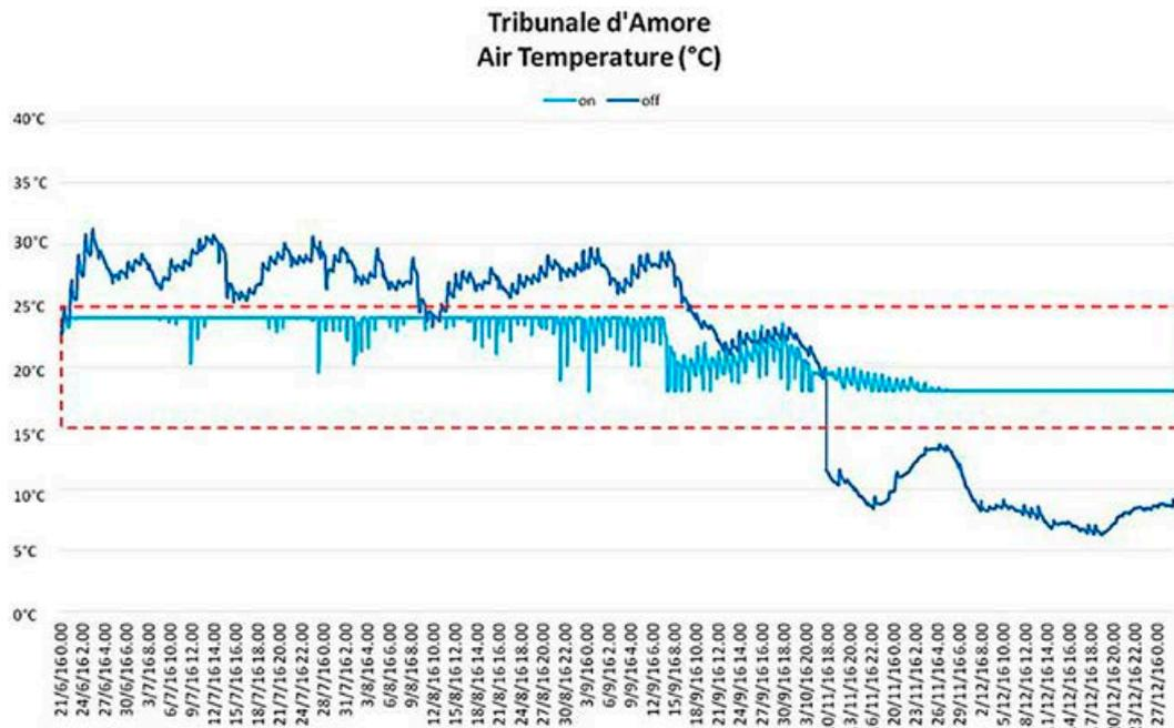
Figure 6. Air temperature trend by building simulation HVAC-ON and HVAC-OFF Scenarios, Room Croce Centrale.
