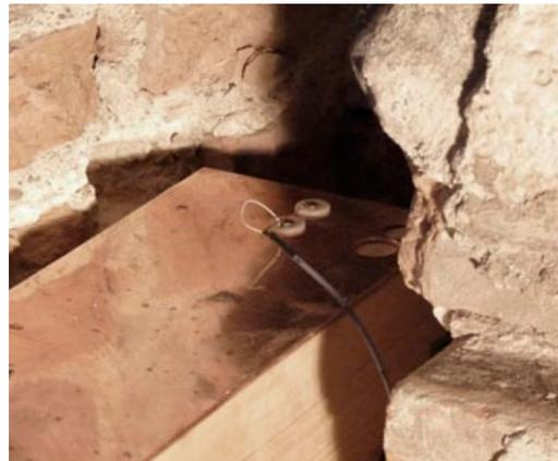
Figure 5. Variant 6 with a copper plate as an artificial thermal bridge. Photo: Fraunhofer Institute for Building Physics IBP.
