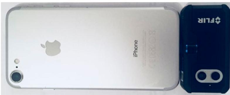
Figure 2. The smartphone (left) and integrated thermal camera (right).
