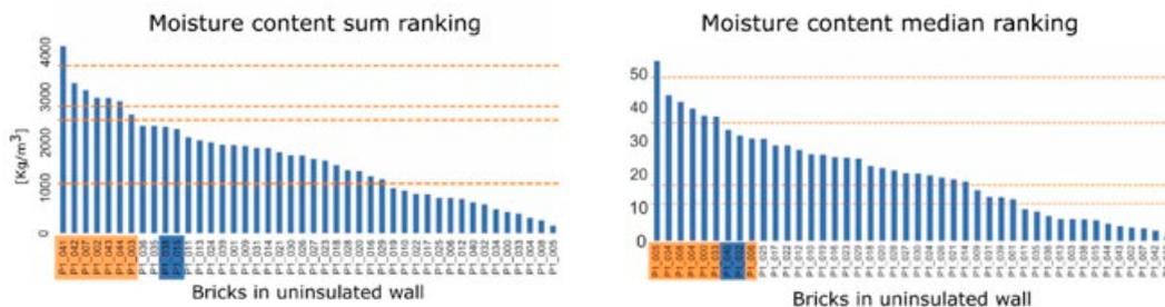
Figure 2. Ranking of bricks based on sum of moisture content (left) and moisture content median (right) at the exterior of a SW oriented  $1\frac{1}{2}$  brick thick wall without insulation. Location Copenhagen, winter 2026–2027 (Dec 1 to Mar 1). The seven highest-ranking brick types in the sum diagram (left), marked with orange, are in the median diagram (right) mixed with two other brick types marked with blue in both diagrams.
