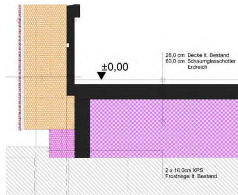
detailed view – insulation from soil
