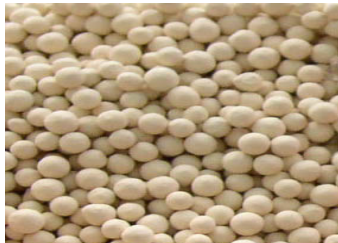
Spheres of zeolite 5 mm, SPF CH
