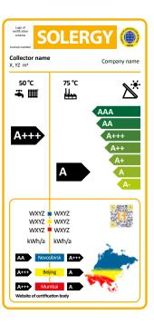
The **SOLERGY label** aims to improve the positioning of solar thermal collectors as generators of CO<sub>2</sub>-free heat, increase transparency about their efficiency, and help consumers make better purchase decisions for an environmentally friendly and sustainable, cost-effective heating supply. It rates solar collectors according to how much solar heat is generated per collector area according to different temperature levels and climate zones.
