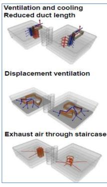
Figure 14 Ventilation system Powerhouse Kjørbo
