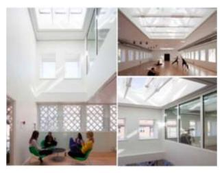
Figur 24 The roof windows have a significant and positive influence on the daylighting level in the building
