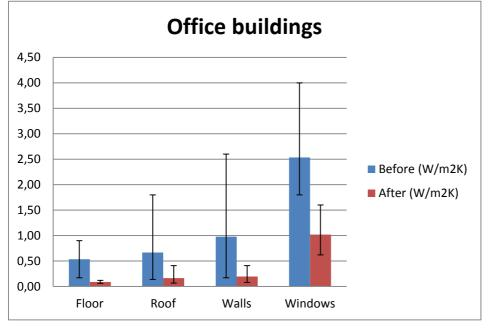
None of the office buildings had insulation added to the ground slab. The Rockwool building and the TU Vienna Plus house implemented measures for the part of the floor which was exposed to air and the figure 10 includes these values. The Rockwool building improved the U- value in the part of the floor that is adjacent to the parking deck, from 0.17 to 0.06 W/m<sup>2</sup>K (between 300 and 750 mm mineral
