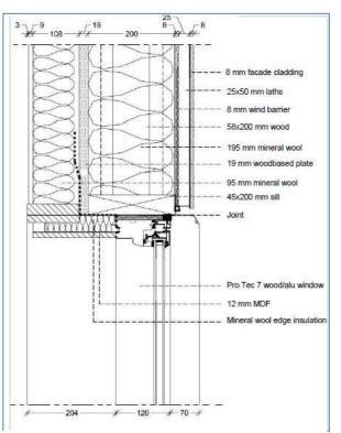
Figure 7 Kindergarten Vejtoften: Cross section of window/wall joint
