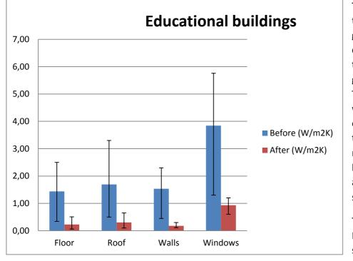
The figure shows that the windows have the greatest absolute change in U-value, and the walls have the greatest relative change. The walls were supplied with 120 - 240 mm of extra insulation. Two of the schools have been renovated to passive house standard according to national standards.
