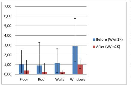
The smallest absolute and relative improvements are in the floors, with a reduction in Uvalues of 58 %. This is partly because of the historic buildings with no changes in the U-values of the floors. Also for the office buildings, the lowest absolute improvement was in the floors. This is the most difficult building component to improve, due to restriction in floor height. In one case, vacuum insulation was used.
