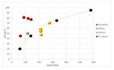
Figure 4 Savings and costs of energy efficiency measures. EU-report: "The energy efficiency investment potential for the buildings Environment; ECORYS/ECN Nov.2012"
