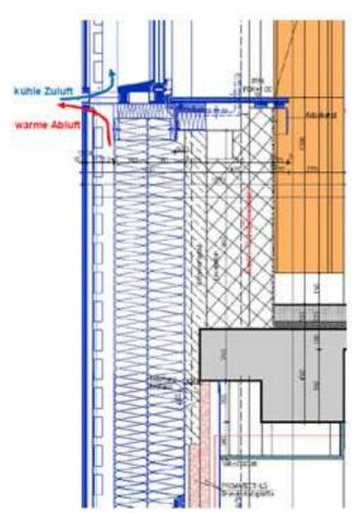
The *TU Vienna Plus Energy building* implemented measures for the roof, the walls, windows and the floor that is exposed to air. An example of a wall with PV panels is shown in the picture. The wall consists of a render (10mm), light-weight concrete (325 mm), a concrete compound (105mm), an air proof barrier (2 mm), a facade insulation wall panel (180 mm), a facade insulation wall panel (160 mm), a wind proof barrier (130 mm) and glazing including a PV- module (13 mm).
