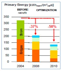
Figure 20 Reduction in primary energy performance, Printing Workshop and Office building energy flow within the system and between the buildings. In the new building there is a cold water storage installed to buffer energy in related temperature levels. Both buildings will be the first step of an overall integrated energy grid of all Fraunhofer campus buildings.
