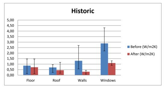
Figure 21 Average, minimum and maximum U-values (W/m<sup>2</sup>K) for the historic and protected buildings
