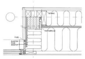
Figure 12 New facade, u-value 0,08 W/m2K, Rockwool
